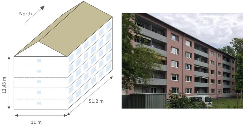
Fig. 4: Geometry and photo of the studied building in Karlsruhe-Durlach.
